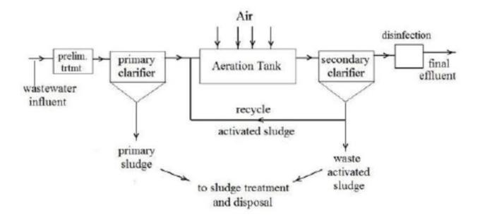
1. Preliminary treatment: waste water contains floating suspended solids such as rags, woods, metals, plastic etc. These have to be removed by screening or other mechanical equipments.
