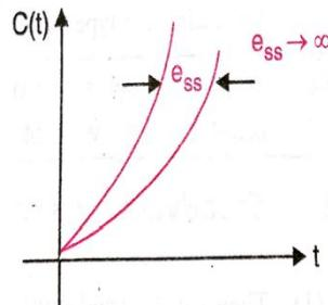
There is infinite steady state error indicating failure to track a parabolic input in type one system
