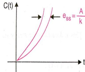
There is finite steady state error for type two system
