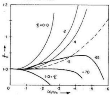
It is seen that for ε =0.7, there is complete linearity for accelerometer for ω/ω<sub>n</sub> ≤ 0.25. Thus the instrument with 100 Hz natural frequency will have a useful frequency range from 0 to 26 Hz at ε =0.7 and will provide very accurate results. For this purpose electromagnetic type accelerometers are widely used nowadays.
