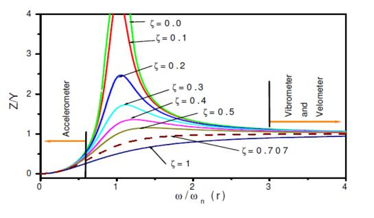
From figure, it can be seen that for large values of  $\omega/\omega_n = r$ , the ratio Z/B approaches unity for every value of damping. The phase angle plot shown below indicates the phase lag of the seismic mass with respect to vibrating base of machine
