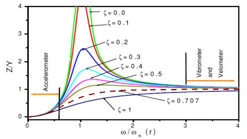
From figure, it can be seen that for large values of  $\omega/\omega_n = r$ , the ratio Z/B approaches unity for every value of damping.
